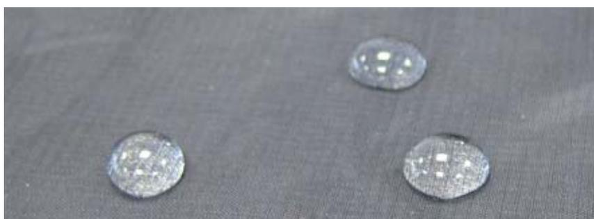
Nylon fabric treated with a water repellent, easy-to-clean coating based on liquid glass.
