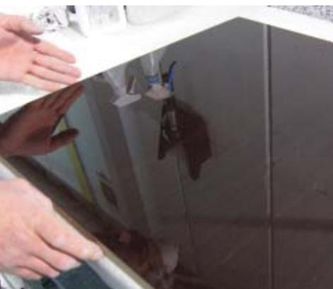
Polished surface of an MDF panel with a bamboo top-layer, treated with a high scratch resistant lacquer based on Nano-SiO<sub>2</sub>.
