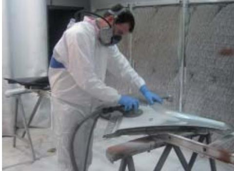
FIGURE 3. Two examples of exposure control measures to prevent exposure to MNM while sanding or polishing MNM containing materials. Left: a vacuum exhaust ventilation workbench; right: optimum protection using nitril gloves, a Tyvek suit and respirator mask with FFP3 filter.
